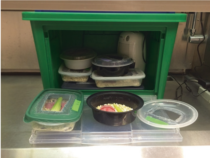
Fig. 1 Beetle housing conditions in the laboratory. In this setup, a front opening box is used as an “isolator,” and individual “batches” of beetles loaded with HDCs are kept in food-quality containers modified with wire screens to allow air to circulate in each batch. A dehumidifier is visible in the back, right of the container. The four batch containers and dehumidifier are resting on a mealworm nursery container (bottom of isolator), where mealworms are allowed to pupate and mature to adults
